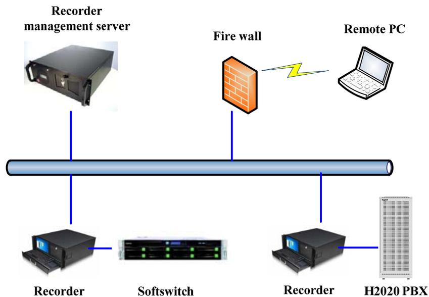
The audio/video recording management server means the unified management functions for the subordinate recording system, which can collect information from the subordinate recording system, and do corresponding statistics according to the requirements, which can also dock with the general network management data, so that the general network management can collect the data and do data statistics on the audio/video recording server.
