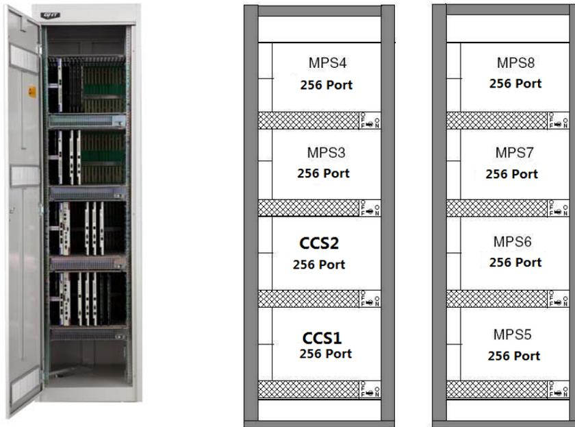
The maximum capacity of the CCS System is 2048 ports. The CCS System is made up of 8 layers of shelves at most. Layers 1&2 are two main control shelves (CCS) and Layers 3 to 8 are subscriber shelves (MPS). All the shelves can be configured with two power modules (PSM) used for redundant power source. Every rack is power-supplied with -48VDC. The CCS System can use redundant or non-redundant public control configuration as per application requirement.
